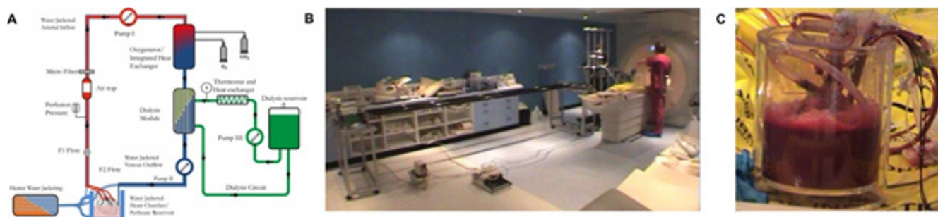
Figure 1 A Scheme of the isolated perfusion mode. Starting from the perfusate reservoir (38°C) the perfusate is firstly passed through the roller pump 2 into a dialysis module and further through a blood oxygenator with integrated heat exchanger. The oxygenated blood is then pumped into the heart via roller pump 1. Before entering the heart an air trap removes air bubbles from the perfusate. The dialysate (38°C) is pumped through the dialysis module with a centrifugal pump (pump 3, flow of 5 l min -1 ) to exchange metabolites between the venous perfusate and the dialysate. The dialysate is re-circulated in a reservoir. T: sensor for dialysate temperature: O 2 and CO 2 : valves for oxygen and carbon dioxide input. The perfusate reservoir and the venous and arterial blood circuits are fully water-jacketed. Temperature is controlled by an external heater. B Detail of the technical setup of the MR compatible perfusion system. All electrical parts (control-unit, power-supply, pumps, etc) are placed approximately 6 meters distant to the magnet. The pump engines were then connected to the custom made MR compatible pump heads using polycarbon tubes. C Detail Heart Chamber
