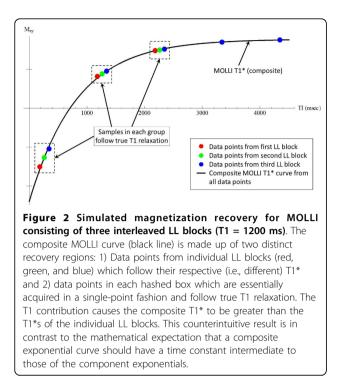
$TI_0$ . In practice,  $TI_0$  is typically too short to completely offset the effects of the LL correction, resulting in the observed systematic underestimation of T1.
